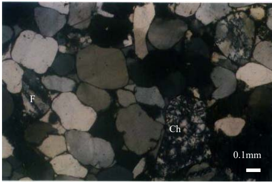
Figure 11. Photomicrograph showing chalcedonic quartz grain (Ch) and weathered feldspar (F) in hard sandstone unit (Between X. N)
