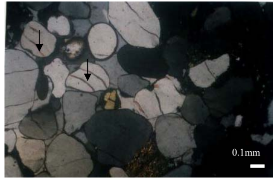
Figure 18. Photomicrograph showing iron oxide fracture filling (Arrow-left) in hard sandstone unit (Between X. N)
