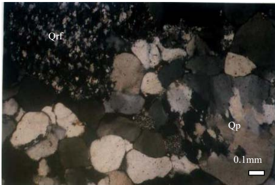
Figure 15. Photomicrograph showing quartzite fragment (Qrf) and polycrystalline quartz (Qp) in hard sandstone unit (Between X. N)
