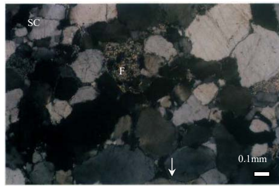
Figure 12. Photomicrograph showing quartz overgrowth (Arrow), weathered feldspar (F) and suture contact in hard sandstone unit (Between X.N.)
