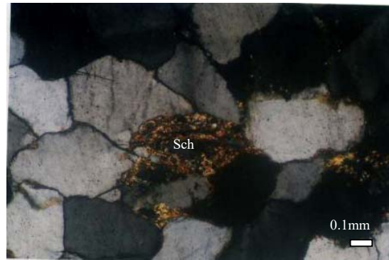
Figure 16. Photomicrograph showing schist fragment (centre) in hard sandstone unit (Between X. N)
