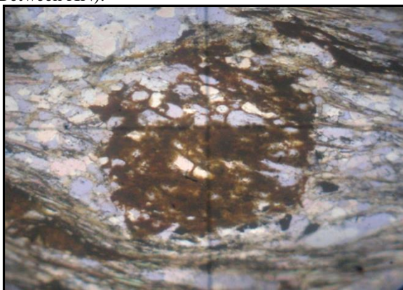
Fig 5: Photomicrograph showing the dominant schistosity of muscovite and graphite. The foliation tends to warp around the garnet porphyroblast due to deformation after they grew (Between XN).
