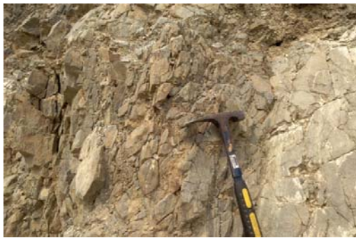
Figure (9). Highly jointed amphibolite that is well exposed near the cart track at south-east of Taungnyo
