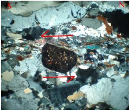
Figure(12).Rotated porphyroblast of garnet indicate N to S left sense of shearing.
