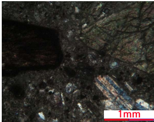
Figure (17). Plagioclase shows polysynthetic twin in hornblende augite andesite
