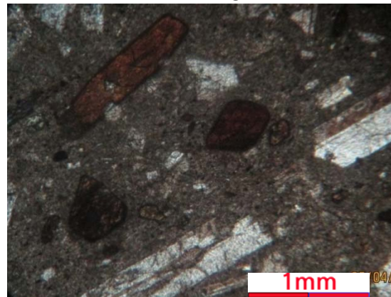
Figure (20). Flow structure occurs in hornblende augite andesite.
