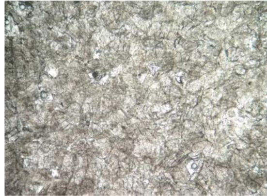
Figure (16) Photomicrograph showing anhedral to subhedral and idiotopic mosaic of the Dolomitized Crystalline Limestone in the Nwabangyi Dolomite Formation Under X.N, 10X
