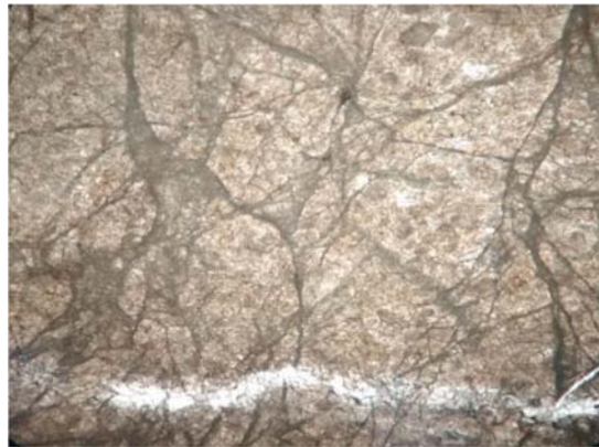
Figure (10) Photomicrograph showing irregular patches & scattered within the micrite with calcite veins of the Dolomitized Dessication Wackestone in the Nwabangyi Dolomite Formation Under X.N.4X
