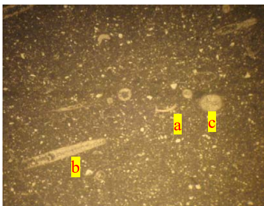
Figure (3) Silty Biomicrite in which thin shell bivalve (a), longitudinal section, (b) and transverse section (c) of tentaculitids and quartz grains are scattered in the micrite under XN, X.40. (Khinzo Chuang Limestone Member)
