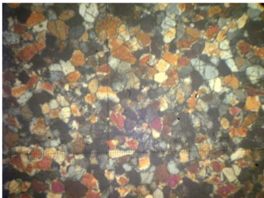
Figure (17). Quartzose sandstone showing subrounded, moderately sorted monocrystalline quartz grains. Under X.N, X.40. (Doganaing Chaung Quartzose Sandstone Member)
