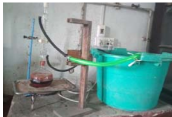
Figure (1). Extraction of cellulose from sawdust by refluxing with sodium hydroxide
