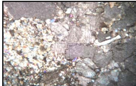
Figure (11). Corrosion of rock fragments in poikilopic calcite cements in protoquartzite (Under X.N 30x).
