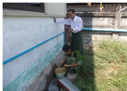
Figure (13). Measurement of the discharge rate at Alpine Purified Drinking Water Factory
