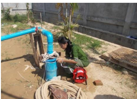
Figure (12). Photograph showing pumping-out test at Alpine Purified Drinking Water Factory
