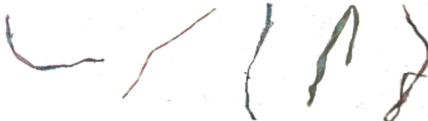
Figure (16). Colorless or blue color and thin slender form of Sillimanite.
