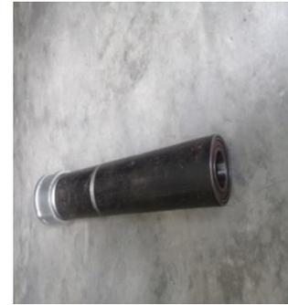
Figure (6). Axial rod of wind turbine
