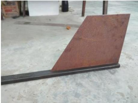
Figure (5). Tail vane of wind turbine
