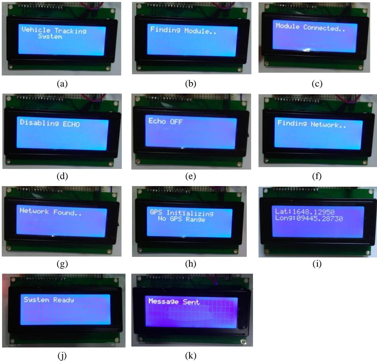
Figurem (8). Display of GPS tracker working functions on LCD
