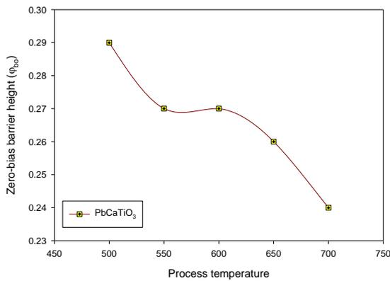
Figure (5). (e) Process temperature dependence of the zero-bias barrier height of PCT thin film
