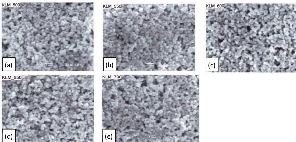
Figure (3). Surface morphology of SEM image of PCT/Si; (a). 500° C, (b). 550° C, (c) 600° C, (d). 650° C and (e) 700° C
