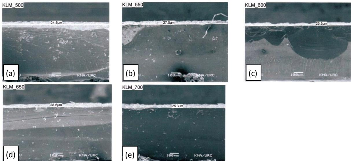
Figure (5). Scanning electron micrograph of cross section of film of PCT heated at; (a). 500° C, (b). 550° C, (c) 600° C, (d). 650° C and (e) 700° C
