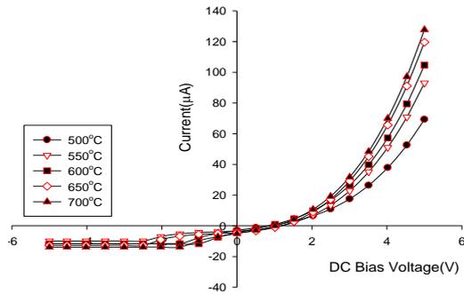
Figure (5). (a) Current and Voltage characteristics of PCT gated FMD with Cu-contact
