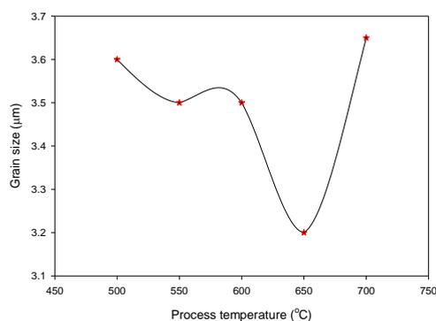
Figure (4). Change in grain size as a different process temperature
