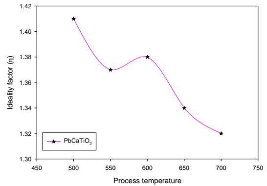
Figure (5). (d) Process temperature dependence of the ideality factor of PCT thin film
