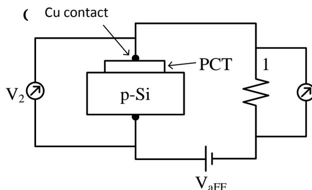
Figure (2). Circuit arrangement for current-voltage (I-V) measurement
