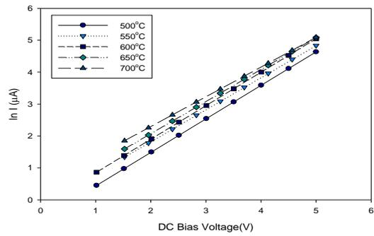
Figure (5). (b) Ln I-V characteristics of PCT gated FMD with Cu-contact
