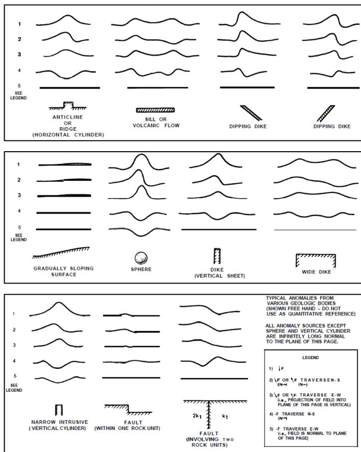
Figure (2). (a), (b) & (c) Anomalies for Geologic bodies at various orientation and different inclinations of the field (after Breiner, 1999).
