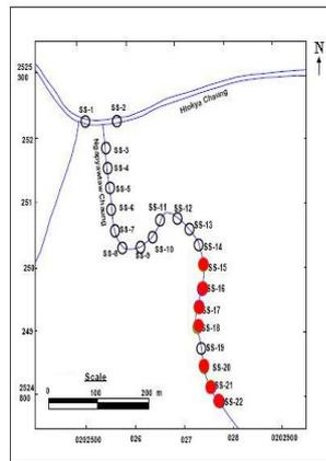
Figure 10. (c). Stream Sediment Anomalies of Silver
