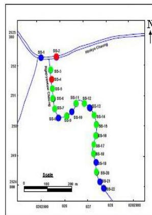
Figure 10. (f). Stream Sediment Anomalies of Zinc
