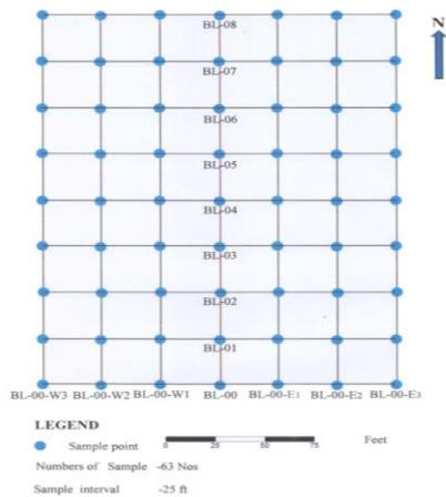
Figure (5). A geochemical soil sampling plan map of Kwinthonze area
