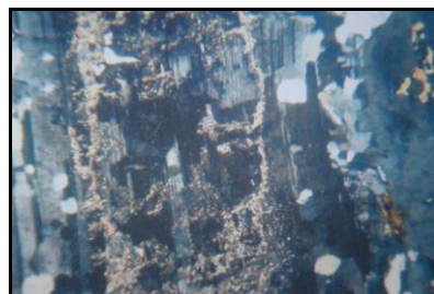
Figure (10). Sericitization along the twin plane of plagioclase feldspar in granite gneiss (Between X.N) (Loc: 037187)
