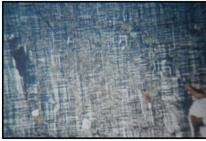
Figure (19). Microcline showing cross-hatched twinning in porphyritic biotite granite (Between X.N) (Loc: 069188)
