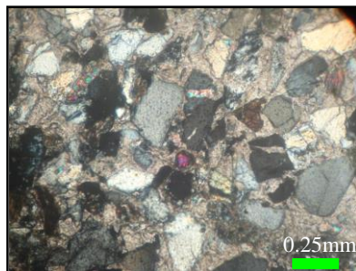
Figure (4). Photomicrograph showing subangular to sub-rounded in shape of quartz grains in Natma Formation (between X.N) (Loc. 875023)
