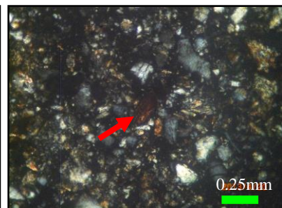
Figure (12). Photomicrograph showing the iron oxide (hematite) develop within biotite cleavage planes (arrow) (between X.N) (Loc.833998)
