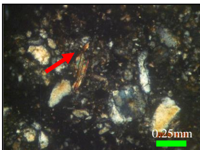
Figure (10). Photomicrograph showing the broken muscovite mica (arrow) by compaction effect (between X.N) (Loc. 841001)
