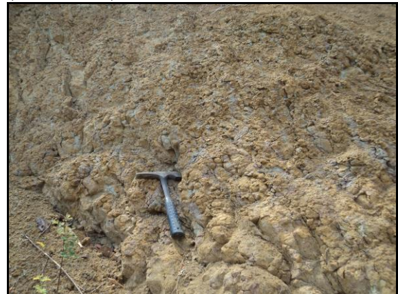
Figure (17). Photograph showing mottled and variegated silty clay indicate semi-arid floodplain paleosols (Loc.885026)
