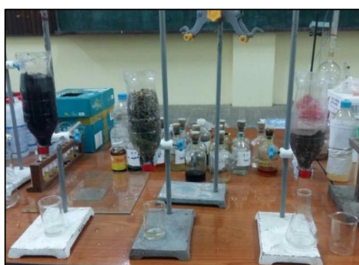
Figure (7). Remediation of arsenic in tube-well water with the various adsorbents by column type method
