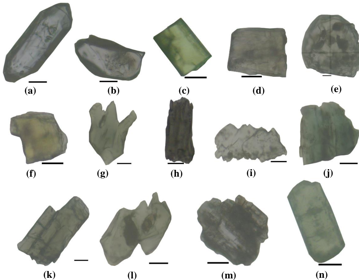
Figure (6). Some heavy mineral occurred in the Naunggauk area (a & b) zircon, (c) tourmaline, (d) rutile, (e) garnet, (f) epidote, (g & h) hornblende, (i) tremolite, (j) hypersthene, (k) enstatite, (l) titanite (sphene), (m) kyanite and (n) olivine (scale bar is 500 \mu m).
